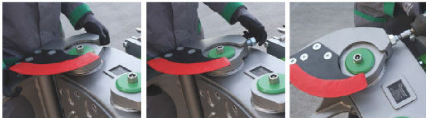
Replacement by hand, fix with locking screw
