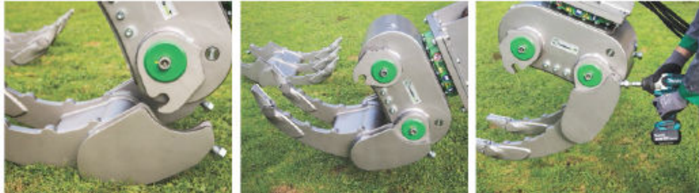
Replacement by hand, fix with locking screw
