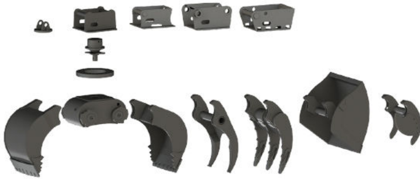
Modular concept design of the grapple assembly
